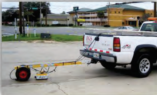
800 MHz GPR Antenna on Road Trailer
